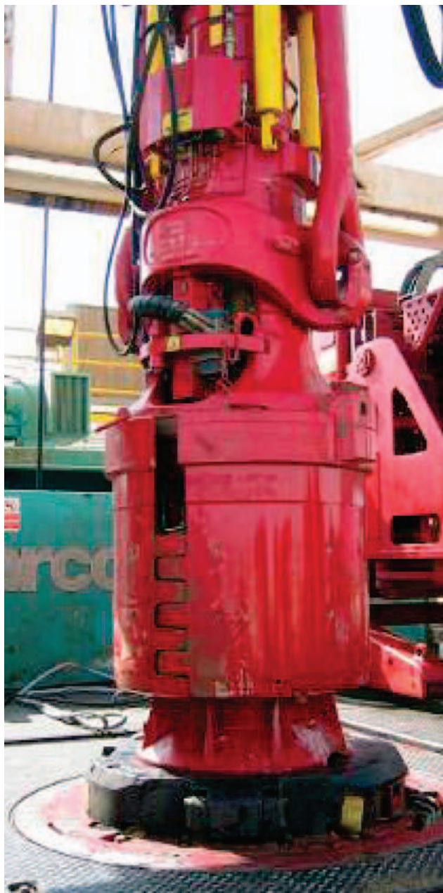
The casing running tool combines features of the top drive, flush mounted spider and conventional casing running tools to result in safer and more efficient operations. It eliminates stabbing board operations, requires less manual handling and eliminates drill floor work platforms. The power casing tong operations have been removed, providing more work space around the well center.
