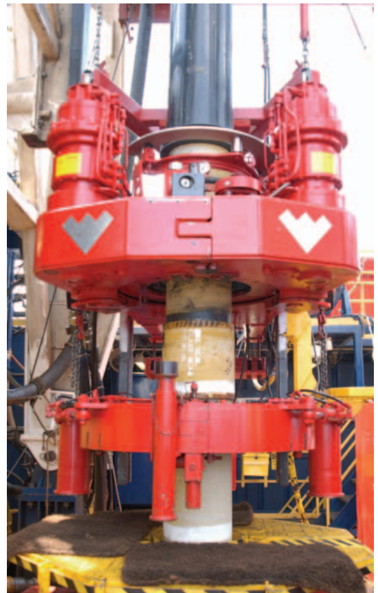
Weatherford's 21-300 power tongs were also installed on Murphy's Front Runner spar in the Gulf of Mexico.
