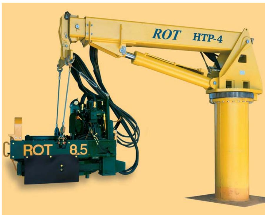
Rogers Oil Tools' automated drill pipe tong technology is fully automated and provides hands-free operation with Cyber-Eye technology that allows the tong to locate the seam of the drilling connection, which is always a constant as opposed to the upset. The HTP-4 free standing pedestal positioning device eliminates rig floor tracks, resulting in greater safety.
