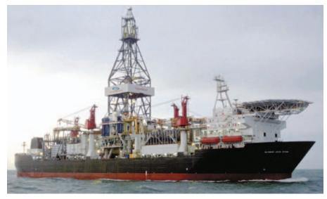
GlobalSantaFe's drillship GSF Jack Ryan, rated for 8,000 ft of water, is drilling for BP offshore Angola under a one-year contract with two six-month options. A potential shortage of drillships in the region could result in dayrates increasing from levels already in the high \$200,000 area.
