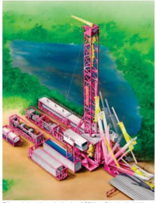
The LOC250 has been This rendering shows the Land and Offshore Containerized 250 ton hookload rig LOC250 in the land configuration. The rig has been designed to drill with conventional drill pipe as well as with casing while drilling technology using the same automated pipe handling and tripping processes.
