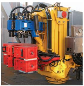
The novel hydraulic iron roughneck is mounted stationary on the rig floor, eliminating the rails typically used with iron roughnecks and resulting in increased safety.
