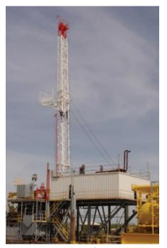
Equipment on Basic Energy Services' Rig 11, the first of the company's three inland workover barges, was completely refurbished earlier this year. The barge can work in up to 10 ft of water and drill to 25,000 ft.
