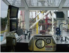
The drillers on Orion's rigs work in climate controlled cabins and perform the drilling operations with joystick controls. The rig is also monitored with Varco's Electronic Driller.
