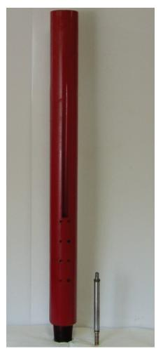
The Downhole Air Diverter has been able to increase the efficiency of the compressed air system, improving drilling performance in most situations where pneumatic fluid is used for cuttings removal.
