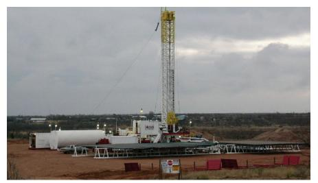
Capstar Drilling's Rig 19 is the newest in its fleet having been delivered earlier this year. Like the company's other rigs, Rig 19 features designs that include a top head drive drilling system and a hydraulically operated pipe handling boom.
