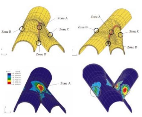
SPE/IADC 52873: This paper describes finite-element work undertaken to assess the effects of internal and external pressure on a sealed multilateral junction. The simulation showed that an unreinforced junction with lateral inclined at 2.5° has burst/collapse resistance of less than 20% of the original casing string. Other simulations were run to determine how to improve these results, for instance by firmly cementing the junction.
