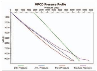
The Pressure Profile 2 graph illustrates an actual MPCD well. The inherently smaller annulus in casing drilling allowed a greater frictional pressure gradient along the lower section of the wellbore. Using managed pressure drilling, a less-dense mudweight was used and the circulation rate was designed to balance the bottomhole pressure while keeping the uphole wellbore pressure below frac gradient. This technology blend allowed drillers to drill ahead and eliminate an intermediate casing string.
