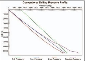
The Pressure Profile 1 shows a well drilled conventionally. A dense mudweight is required to balance the bottomhole pressure but causes the wellbore pressure uphole to exceed the frac gradient. Drillers typically set intermediate casing string to avoid hole collapse, lost circulation or loss of hole. These profiles were created using the Hydraulic UnderBalanced Simulator developed by Signa Engineering Corp.
