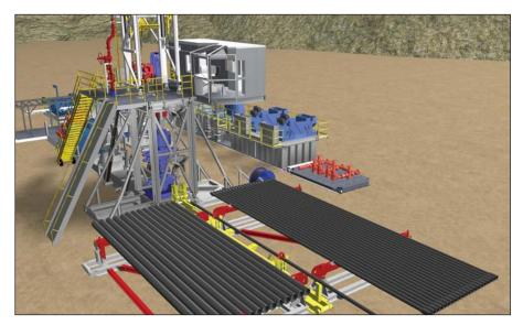
Computer renderings demonstrate the concept of National Oilwell Varco's Rapid Rig, debuting this month. The rig was designed to be small and easy to move, making it suitable for drilling programs with shallow to moderate depths of 6,000 to 10,000 ft.
