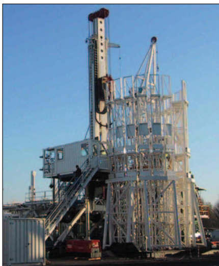
The Italian-built Drillmec HH 300 hydraulic rigs feature an automated pipe handling system based on a vertical basket, top drives, touch screen digital controls and are rated at 1,500 HP.
