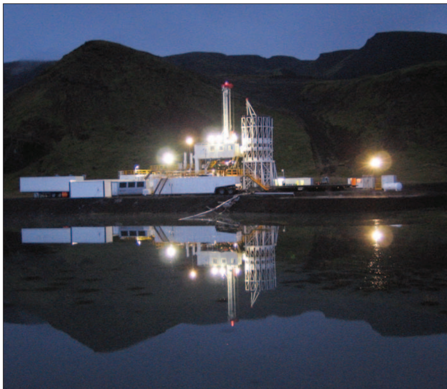
The Italian-built Drillmec HH 300 hydraulic rigs feature an automated pipe handling system based on a vertical basket, top drives, touch screen digital controls and are rated at 1,500 HP.
