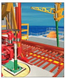
Above: Gun module in rotary and gun module being handled by automatic rig handling equipment. Below: Iron roughneck making up 2 gun modules, with bottom of the gun connector stabbing into top of gun connector. Left: Quick Torque Connector Sub-Assembly.
