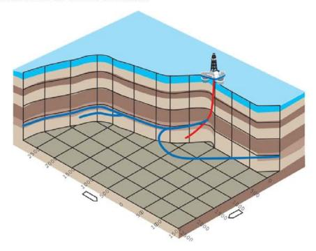
The multilateral wells in Hydro's Troll field in the North Sea were steered to within 1/2 meter of accuracy along very long horizontal lengths in order to optimally penetrate the very thin formation, requiring continuous and precise geosteering to remain within the optimum pay.
