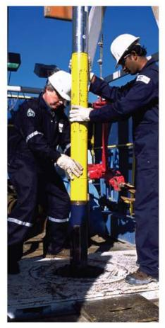
Smaller OD RSS technology such as Baker Hughes INTEO's 4 3/4-in. AutoTrak system could offer operators a new enabling technology to extend the life of mature fields.
