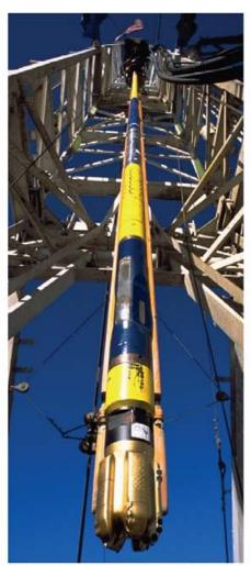
Baker Hughes INTEO's AutoTrak rotary steerable system is a hybrid, incorporating parts of both push-the-bit and point-the-bit steering methods to take advantage of each method's strengths.
