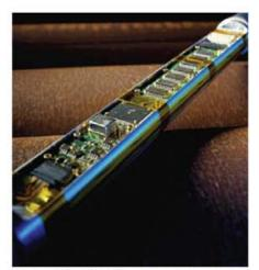
The TrendSET EM/MWD system includes electromagnetic telemetry for underbalanced drilling operations, mud pulse telemetry for mud applications and is application configurable for directional and logging operations. Weatherford is beginning field tests on the dual space propagation resistivity (DSPR) tool for UBO, which also provides accurate resistivity for all fluids.
