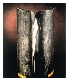
This photo illustrates the amount of casing damage that can occur from the drill pipe tool jointwhen older hardbanding techniques are used, such as tungsten carbide particles applied to the pipe in a raised condition. arguably the most effective wear reduction method ever devised. The hardbanding was applied in a raised (proud) condition. Consequently, the hardbanding accomplished its goal: protect the drill pipe tool joint from rapid abrasive wear.
