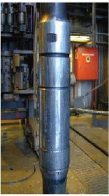
This tool joint has wear-resistant hardbanding applied to reduce wear to the drill pipe and joint as well as reducing wear and damage to casing.
