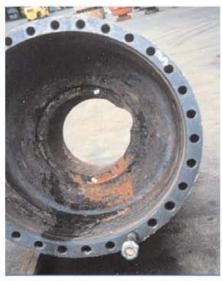
Present hardbanding materials and techniques have eliminated damage to casing. Damage to marine risers like that in the above photo has also been virtually eliminated due to modern hardbanding techniques.
