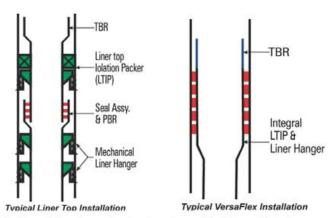
The integral liner hanger/packer, is made up of an integral tieback receptacle above an expandable solid hanger body. Elastomeric elements are bonded on the body. As the body is expanded, the elastomeric elements are compressed in the annular space. No moving parts, slips or cages to suspend the liner in the support casing are necessary. Multiple redundant elastomeric elements maintain pressure integrity while virtually eliminating gas migration paths in the liner top.
