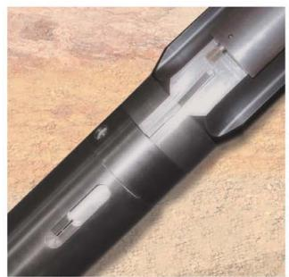
The InForce HCM-A adjustable sliding sleeve can eliminate intervention and associated risks by providing multiposition choking for zonal control to help optimize production or injection. The sleeve has six standard choking positions ranging from 3% to 20% of the full tubing area plus full open and full closed.
