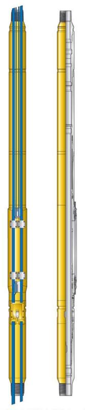
Baker Oil Tools' HCM-A infinitely variable hydraulic choke has been successfuly flow tested with over 300,000 lbs of sand at rates exceeding 25,000 bpd without significant choke wear or seal system damage.
