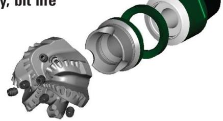
The different components of matrix PDC bit. As opposed to roller cone bits, PDC bits have no moving parts. PDC bits can be manufactured from two different materials, steel bodied and matrix bodied bits.
