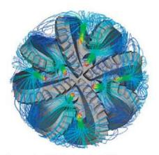
Computational fluid dynamics (CFD) programs enable modelling the fluid flow around bits inside a borehole to investigate bit designs and optimize fluid flow.
