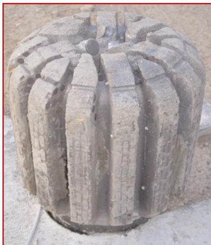
Figure H: The dull condition of the experimental 6 1/2-in. A2 in the Rockies after 360m.
