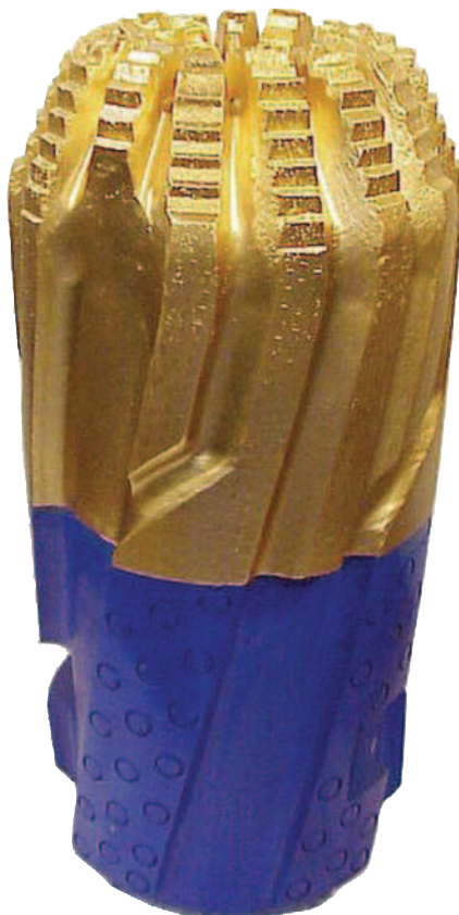
Figure 1: Field experience of historic bit designs had shown that an interrupted blade profile as shown here produced increased penetration rates when operating through interbedded shale containing formations.
