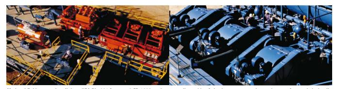
Mud and fluid processing: Nabors USA Rig 304 features 3 FB-1600 mud pumps, all capable of simultaneous operation at the manufacturer's hydraulic horsepower rating. The 4-tank, 2,100-bbl mud system is equipped with a SWACO fluid-processing system and a custom-designed collection tank complete with augers for cuttings transfer. The mud system can be configured for 1,100 bbl, 1,600 bbl or 2,100 bbl simply by switching valves.
