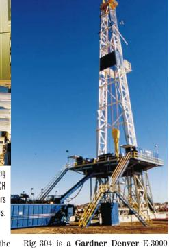
Rig 304 is a **Gardner Denver** E-3000 with a 1,650,000-lb capacity mast and self-elevating substructure. The power package consists of four 3512 B **Cater-pillar** electronically controlled 1,475-hp engines driving 1,505-kw generators to power an IPS 5-bay SCR house.
