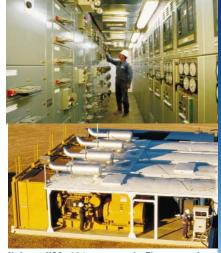
Nabors USA 304 revamped: The sweeping upgrades to this 3,000-hp rig included an SCR system withy programmable-logic controllers (top) powered by four 1,475-hp Cat engines. The rig boasts a 1.65 MM lb capacity mast.
