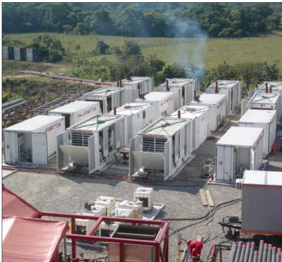
In this MPD project, cryogenic nitrogen was phased out in favor of membrane nitrogen equipment, which provided cost reductions and eliminated logistics concerns with cryogenic nitrogen supplies.
