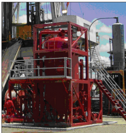
The pressurized separator used was capable of handling surges of up to 50 MMscfd gas/nitrogen, liquid rates up to 35,000 bbl/day, as well as 1,800 bbl/day of drill solids.
