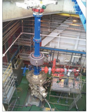
Deck space was an important issue in this Norwegian underbalanced operation, as the surface separation package with the choke manifold and the pumps occupied almost all available deck space in the BOP areas.
