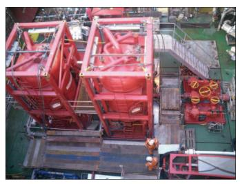
The mobile surface separation system consisted of 2 vessels. In the first stage, the main part of the gas was extracted and routed to the platform high-pressure flare system. Solids were removed, and liquids were routed to the second stage separator. In the second stage separator, any remaining gas was taken out and routed to the platform low-pressure flare system.
