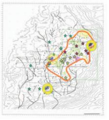
Part of the complex Gullfaks field (shown above) became undrillable with conventional technology. Excessive water injection in the problem area, indicated by the red border at left, caused pressure increases and related fracturing of the reservoir's cap rock.
