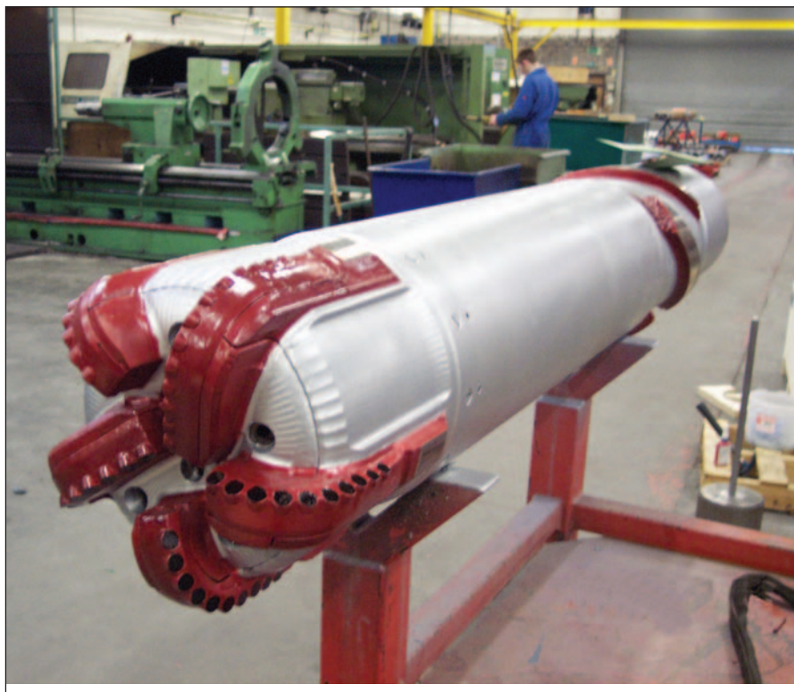
Weatherford’s 9 5 / 8 -in. by 12 1 / 4 -in. DrillShoe III is a displaceable bit used for formations with up to 18,000 psi compressive strength. It has a premium cutting structure that is displaced to the annulus after drilling to TD by a simple pressure cycle.
