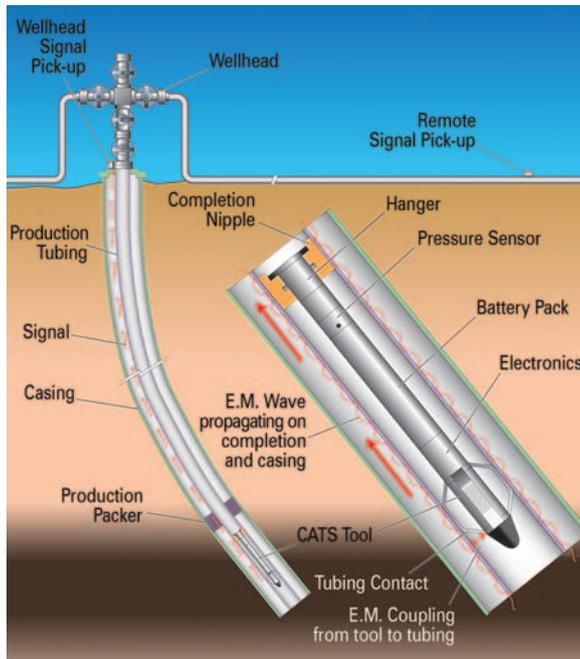
**Expro Group's cableless telemetry system offers an option to high cost downhole data gathering by providing a cost effective alternative to surface read-out data for onshore wells.**
