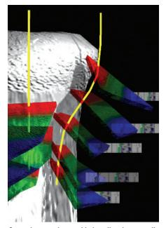
Screenless sand control helps allow better wellbore access than screen based completions. Multiple completions or recompletion of stacked pay zones can be facilitated by open wellbore access.
