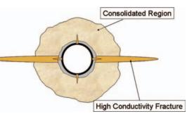
Near-wellbore consolidation and frac stimulation helps stabilize is the formation at the wellbore to minimize sand and fines movement. A tip screen-out frac stimulation using the LSR system Completions on wells with proppant coating improves connectivity of the wellbore to the reservoir for improved productivity. The LSR proppant coating stabilizes the proppant bed to prevent proppant movement and at a later date. Ten or more reduce loss of conductivity by fines plugging.
