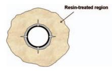
Near-wellbore consolidation stabilizes the formation to help prevent sand and fines production. Testing with reservoir core material shows that the consolidated region can maintain more than 85% of its original permeability.
