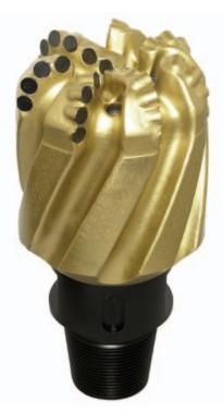
More than 100 PDC bit design iterations were used on the Troll field, leading to improved cutter design and geometry as well as enhanced bit hydraulics and gauge configuration. The current standard bit features 19 mm cutters, seven blades and a 6-in. long gauge.
