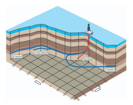
Troll field challenges facing the operator included a thin oil column, dramatic differences in formation drillability throughout the reservoir affecting directional control, and complex long horizontal sections coupled with demanding well profiles.
