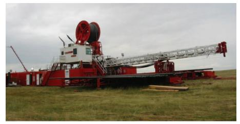
Ensign Resource Service Group's ADR-1000-CT rigs can drill with both jointed drill pipe and coiled tubing. The rigs can drill and case the surface hole with jointed pipe and then drill to TD with coiled tubing. The company ordered ten such units that will be delivered this summer, all of which are earmarked for the Canadian shallow well drilling market.
