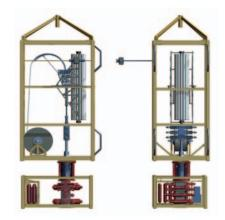
The SIM module includes a bottom hole assembly carousel tool rack that contains different BHAs for a particular job. The BHAs are selected from the tool rack, latched to the end of the coiled tubing and then run into the wellbore. joint venture (SIM Ventures Ltd) comprised of BJ Services and Otto Candies. The joint venture will operate the SIM following design and construction of the vessel and module, expected to occur in 2008.
