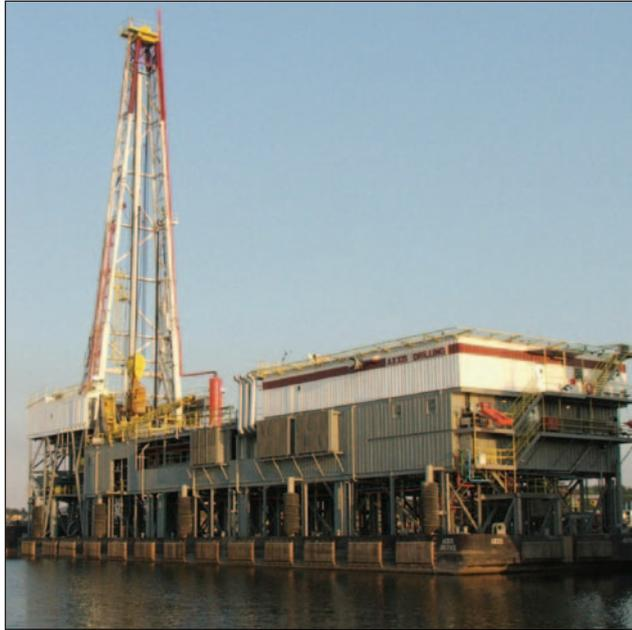
The *Justice*, a 3,000-hp posted barge capable of drilling to 30,000 ft, recently joined Axxis Drilling's fleet, as did the 2,000-hp barge *Liberty*.
