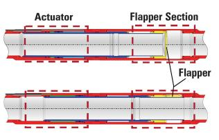
The main challenges to achieve A solution to some of the financial and technical challenges of underbalanced operates has been found in a newly developed technology called the downhole isolation valve (DIV). SPE/IADC 92595.
